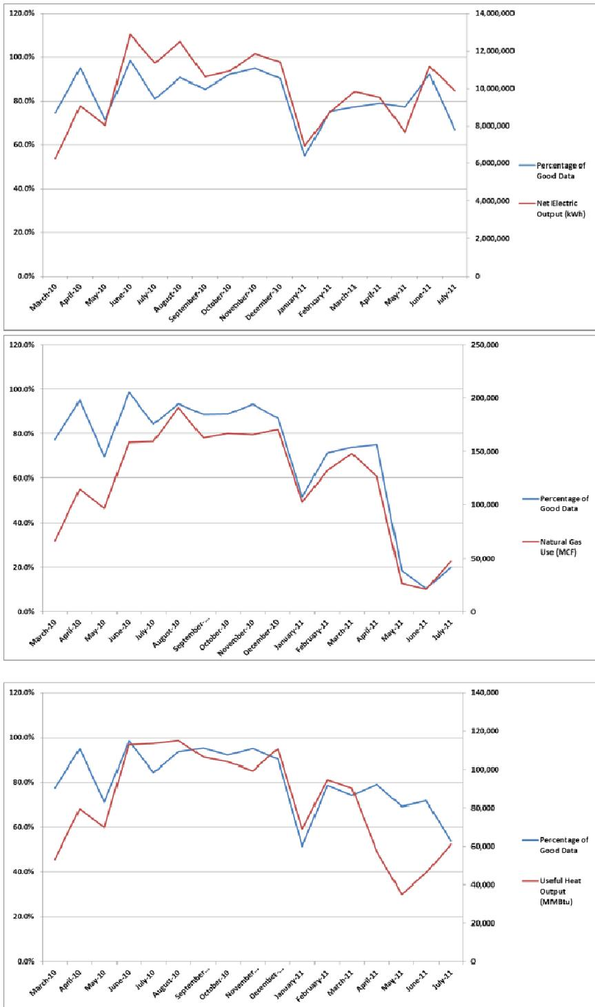
FIGURE 16 CORRELATION BETWEEN DATA QUALITY, KWH, FUEL AND USEFUL HEAT
