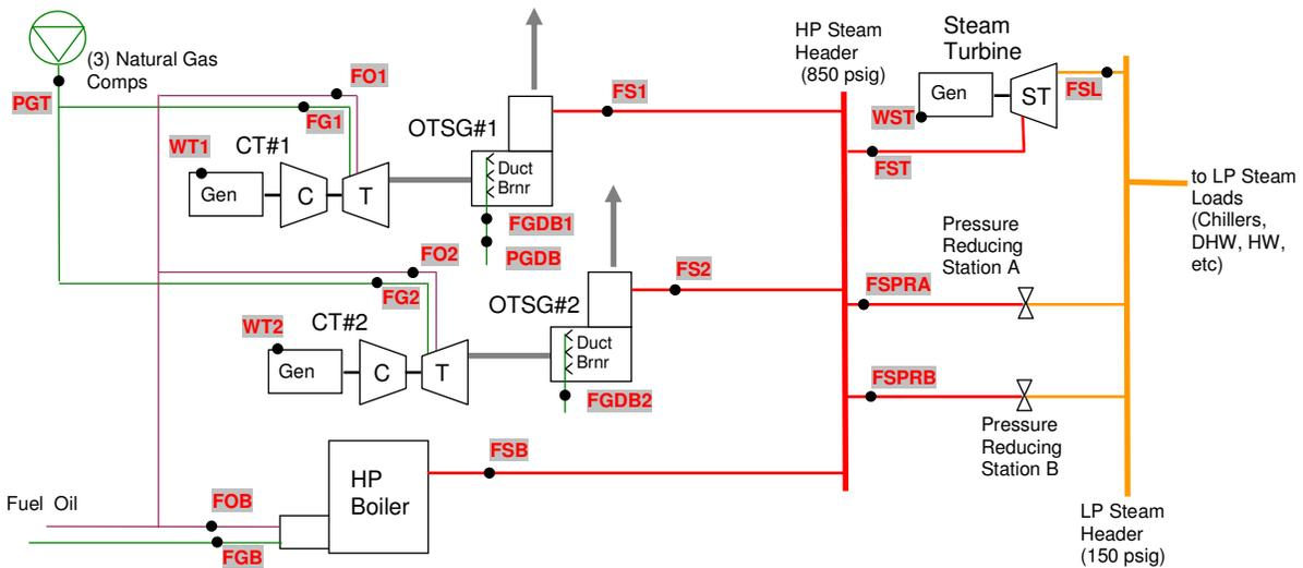
FIGURE 4. SCHEMATIC OF CHP SYSTEM WITH MONITORED DATA POINTS SHOWN
