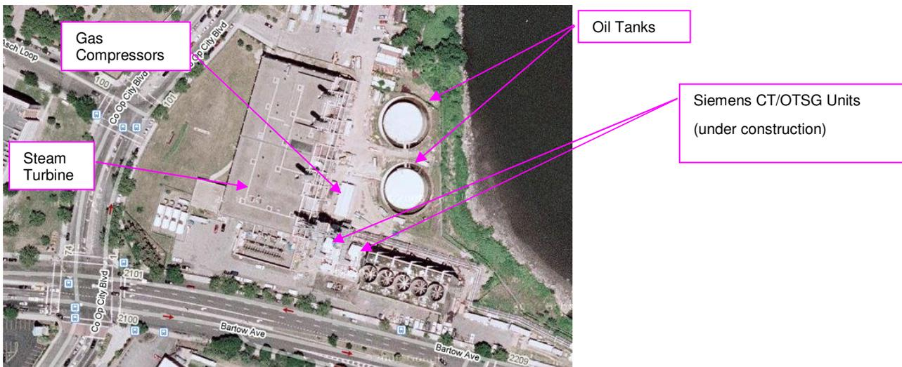
FIGURE 3. SATELLITE PHOTO OF PHYSICAL PLANT AT CO-OP CITY
