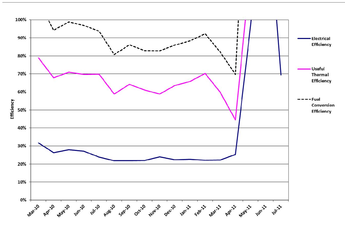
FIGURE 5 CHP SYSTEM EFFICIENCY BY MONTH
