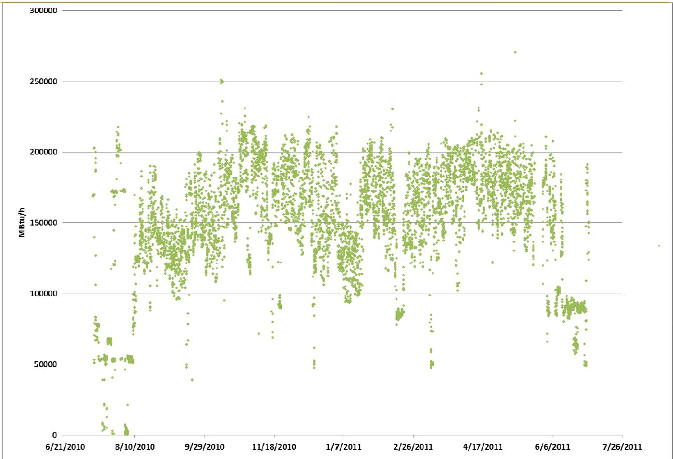
FIGURE 7 CHP USEFUL THERMAL OUTPUT VERSUS TIME
