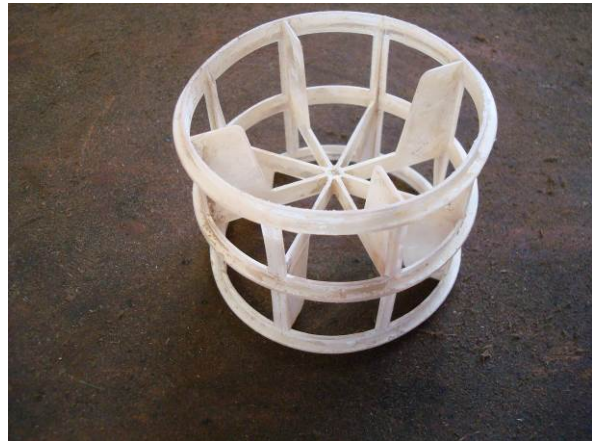
Media on which bacteria grow, located in upper portion of scrubber.
