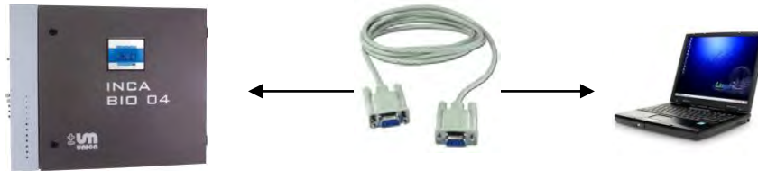
Figure 5-2: Communication between the INCA Analyzer and PC
