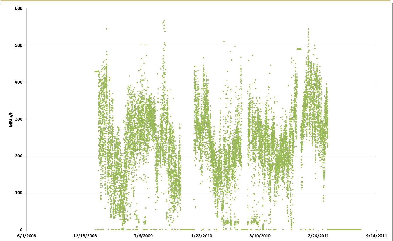
FIGURE 8 CHP USEFUL THERMAL OUTPUT VERSUS TIME
