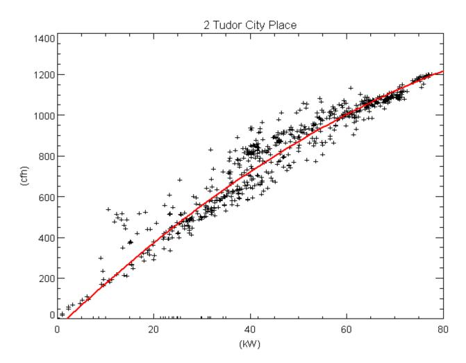
Power generation (WT\_KW), gas consumption (FG):
