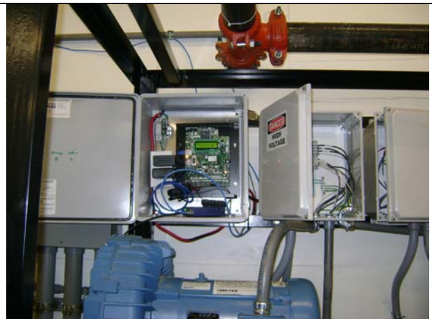
CDH data logger and enclosure (left)
