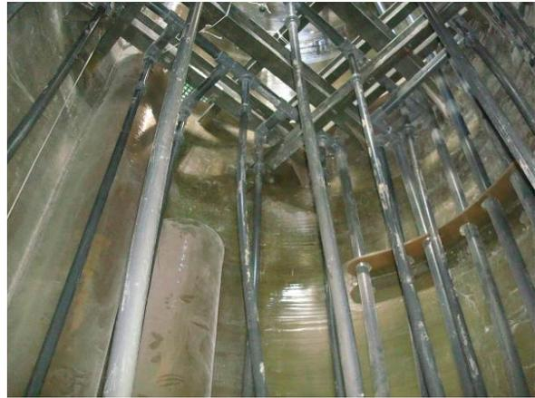
First deck of bioreactor looking up towards second deck (without packing material) – vertical PVC piping for feeding bacteria and rinsing packing material.
