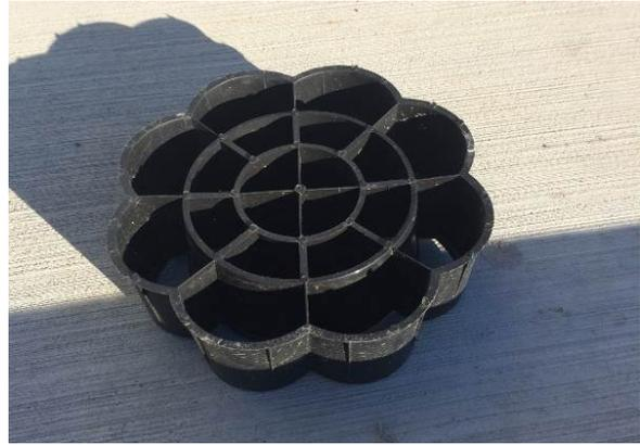
Bioreactor packing material.
